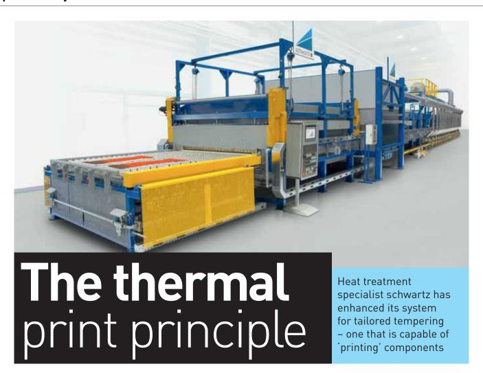
ress hardening has established itself as an exceedingly cost-efficient and versatile-to-employ process for making very strong, yet lightweight, automotive safety components. It has evolved into a standard technology in automotive manufacturing.
